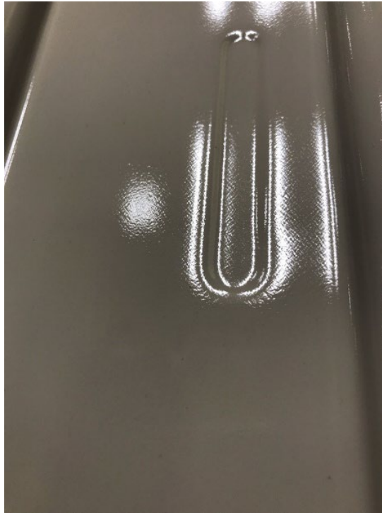
Orange peel in ONTEX® part due to Overheating
