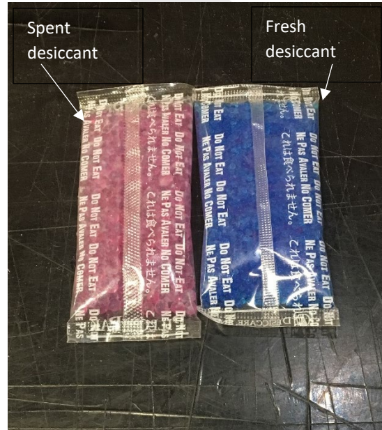
Spent desiccant pack (left) vs. fresh one (right)
