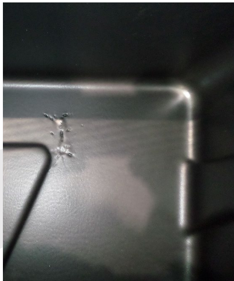
Example of moisture issue in ABS causing an A side defect
