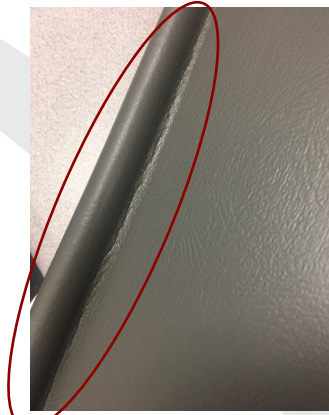
Slight wrinkling into tight radius
