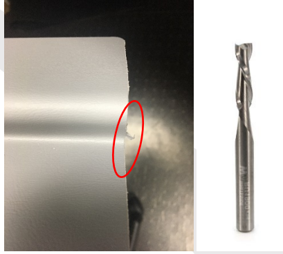
Example of vinyl laminate chaff from routing and an “up flute” bit
